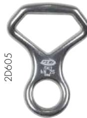
Figure of 8 belay / abseil device for mountaineering and climbing. The squared shape reduces rope twisting and the curved profile allows two different descent speeds.
