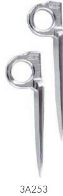
Soft steel zinc plated piton with V tip. To be used on soft rock (limestone etc.). It deforms adapting itself to the cracks of the rock.
